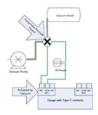
Take care to ensure that the wire connections are made fast, and the voltage and current does not exceed 250V or
