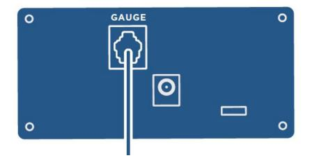
The Display controller can be connected to a computer with a standard micro-B USB cable. The software will automatically download and install. You can open a simple command window like <u>putty</u> and issue commands to read vacuum and assign set point values.
