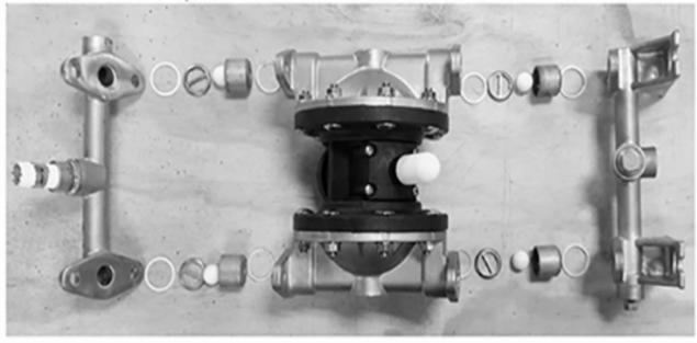
This is how the stainless steel valve body goes together. The tapered edges will always seat against the white plastic seals. The white plastic seals will always be nested against the bottom of the bore of the diaphragm body and against the upper and lower manifolds.
